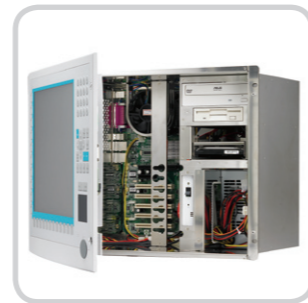
IPPC-7000's detachable sideopen front panel
