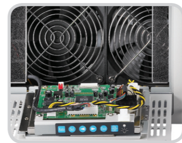
Dual fan & modular LCD kit with OSD
