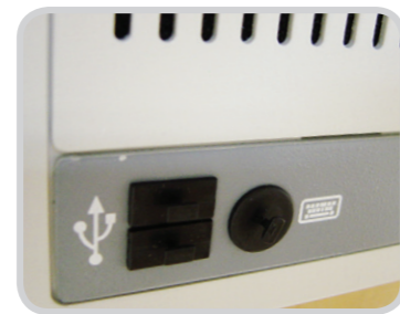
Front-accessible USB 2.0 & PS/2 ports
