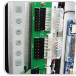
OSD control behind the front panel of IPPC-7000 series
