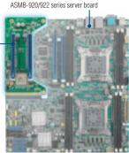
Advantech's PME (Powerful Modular Expansion) design allows versatile expansion module options to the ASMB-920/922 series motherboards. PME expansion cards are an economical, effective solution for a range of applications, providing function expansion for a range of PCle modules. In addition to meeting standard industrial specifications, Advantech's PME modules fit just about anywhere. They are easy to assemble and provide a simple upgrade path.
