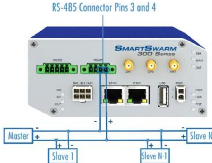
NOTE: this device will only operate in Passive (receive-only) mode. It is not possible to configure it as a Modbus Master, or for it to transmit on the Modbus network.
