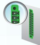
Built-in DI/DO for simple I/O control, status detection, lighting control and event triggering in order to save extra cost and devices.
