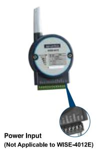
The WISE-4000 is designed for a standard industrial unregulated 24 VDC power supply. For further applications, it can also accept 10~30 VDC of power input, 200mV peak to peak of power ripple.
